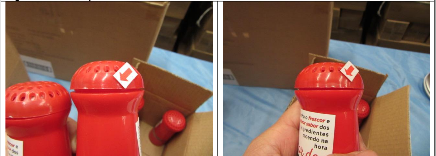
Remark 6: For item# CV150897 and CV150898, found 80% of inspected samples with outstanding gap between parts due to poor assembly.
