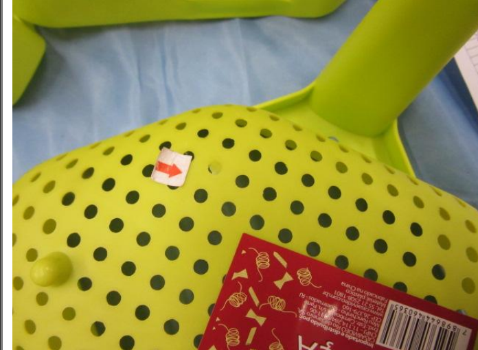
Remark 7: For item# CV150906 and CV150907, found 100% of inspected samples with one or more holes that did not penetrate.
