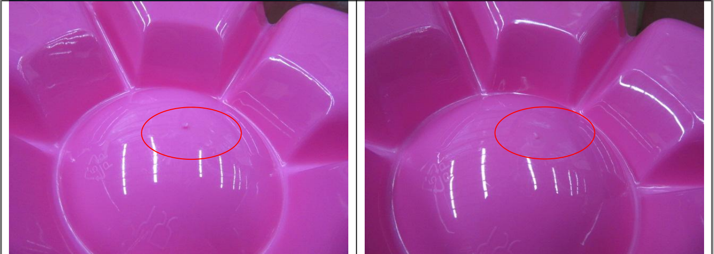
Remarks 5: For item# CV150899 and CV150900, found 70% of inspected samples with untrimmed flashing at gate on bottom of product.
