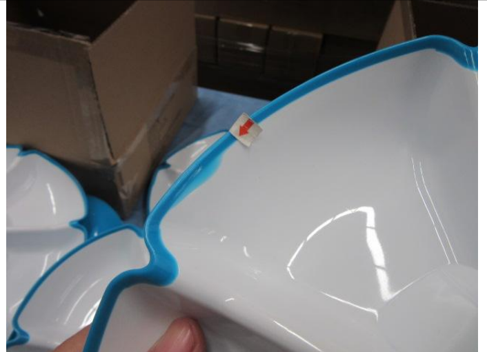
Poor painting on housing-Minor
