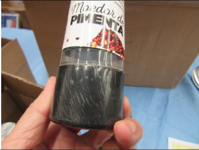
Poor painting on housing-Minor
