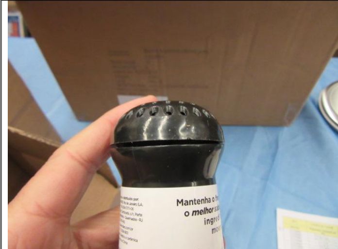
Remark 6: For item# CV150897 and CV150898, found 80% of inspected samples with outstanding gap between parts due to poor assembly.
