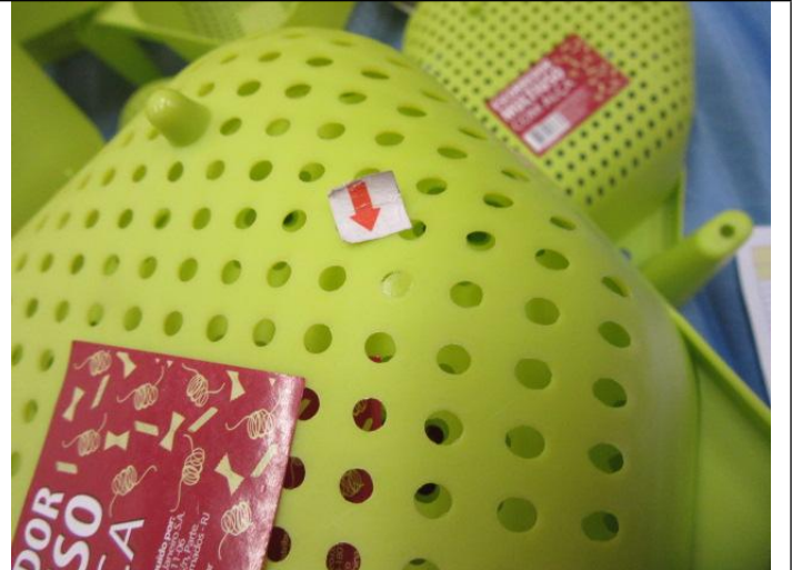
Remark 7: For item# CV150906 and CV150907, found 100% of inspected samples with one or more holes that did not penetrate.
