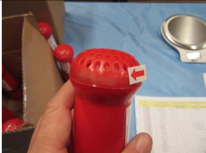
Poor painting on housing-Minor
