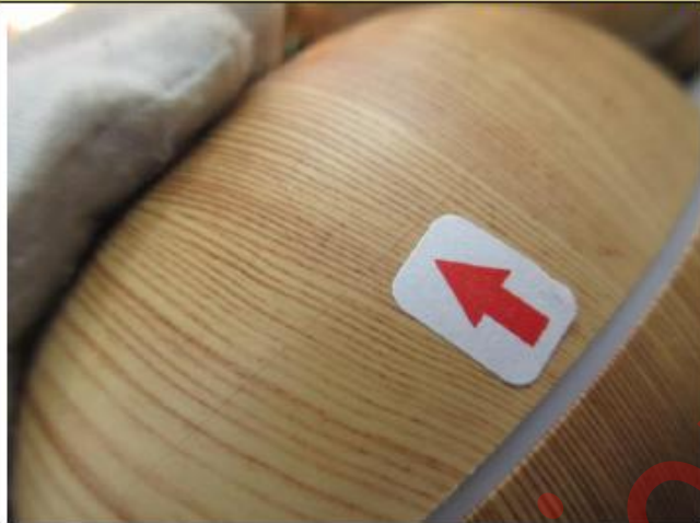
Scratch on housing--Minor
