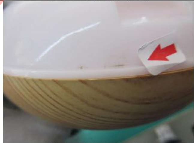
Dirty mark in housing--Minor
