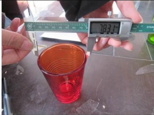
Remark 2: The actual size of the cup was 7.8-7.9cm X 10.3-10.5 instead of 8.2cm X10.5cm given by client.
