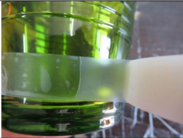
Adhesion Check for Coating
