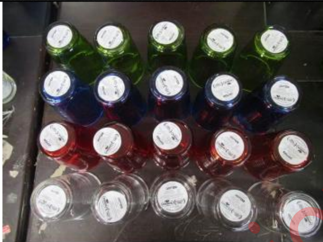
Remark 3: Found 10%of the sample size,the bottom label was more or less skew.
