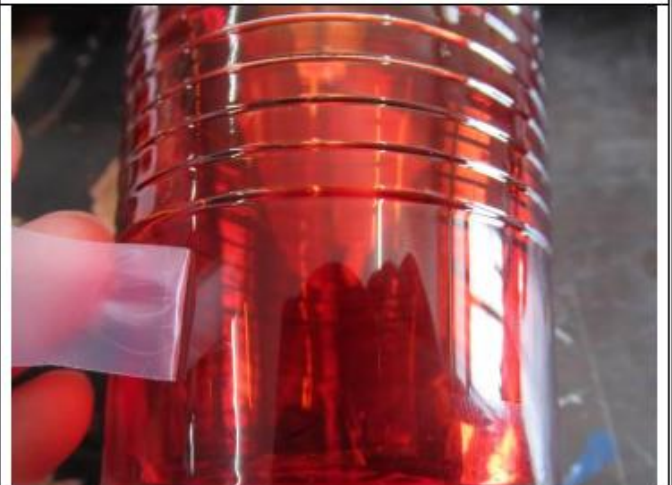
Adhesion Check for Coating
