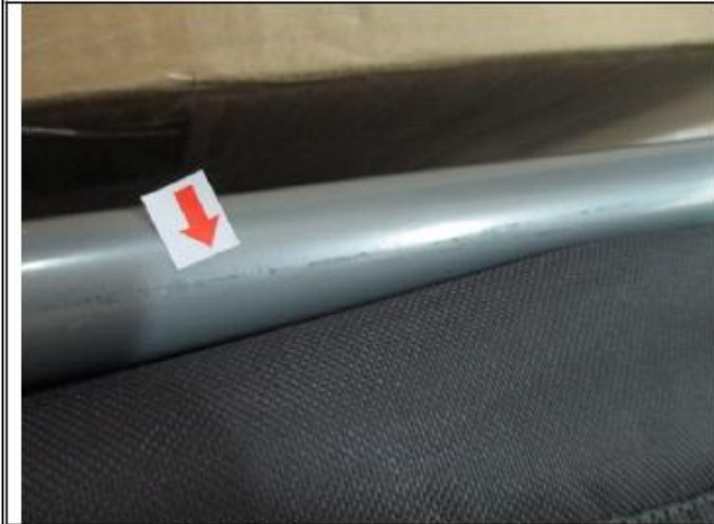
Scratched mark on the surface major
