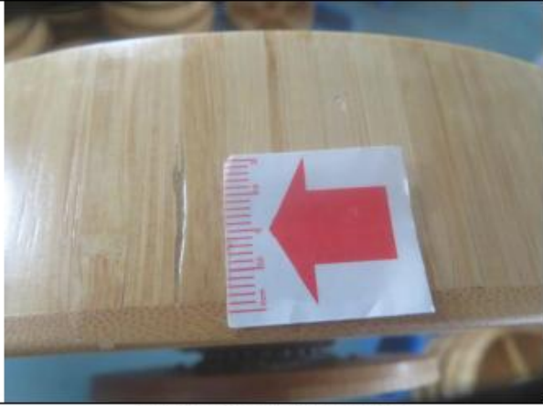
Lack of materials-Minor
